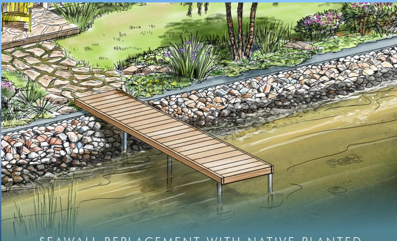
SEAWALL REPLACEMENT WITH NATIVE-PLANTED BUFFER STRIP BEST MANAGEMENT PRACTICE
